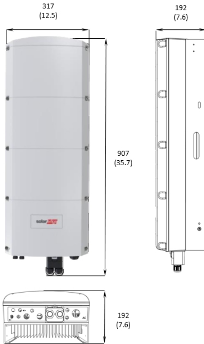
Figure 29: SolarEdge Home Hub Inverter - Three Phase: dimensions
